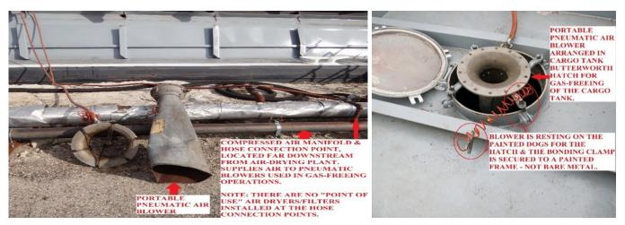
Not installing "point of use" air dryers/filters at hose connection points for pneumatic air blowers (left photo) & attaching air blower bonding clamps to painted surfaces instead of bare metal (right photo) can lead to dangerous static build up.
